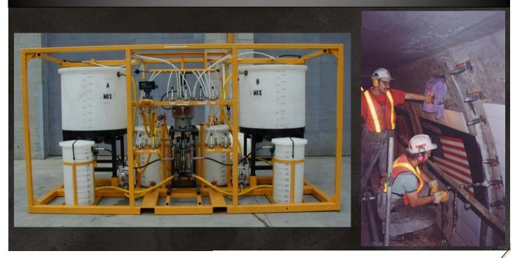
Chemical grouting can be used to stabilize soils for tunneling, control water seepage, and provide excavation support. Chemical grout is injected under pressure in order to permeate soils and create a homogenous mass with increased strength and reduced permeability.
