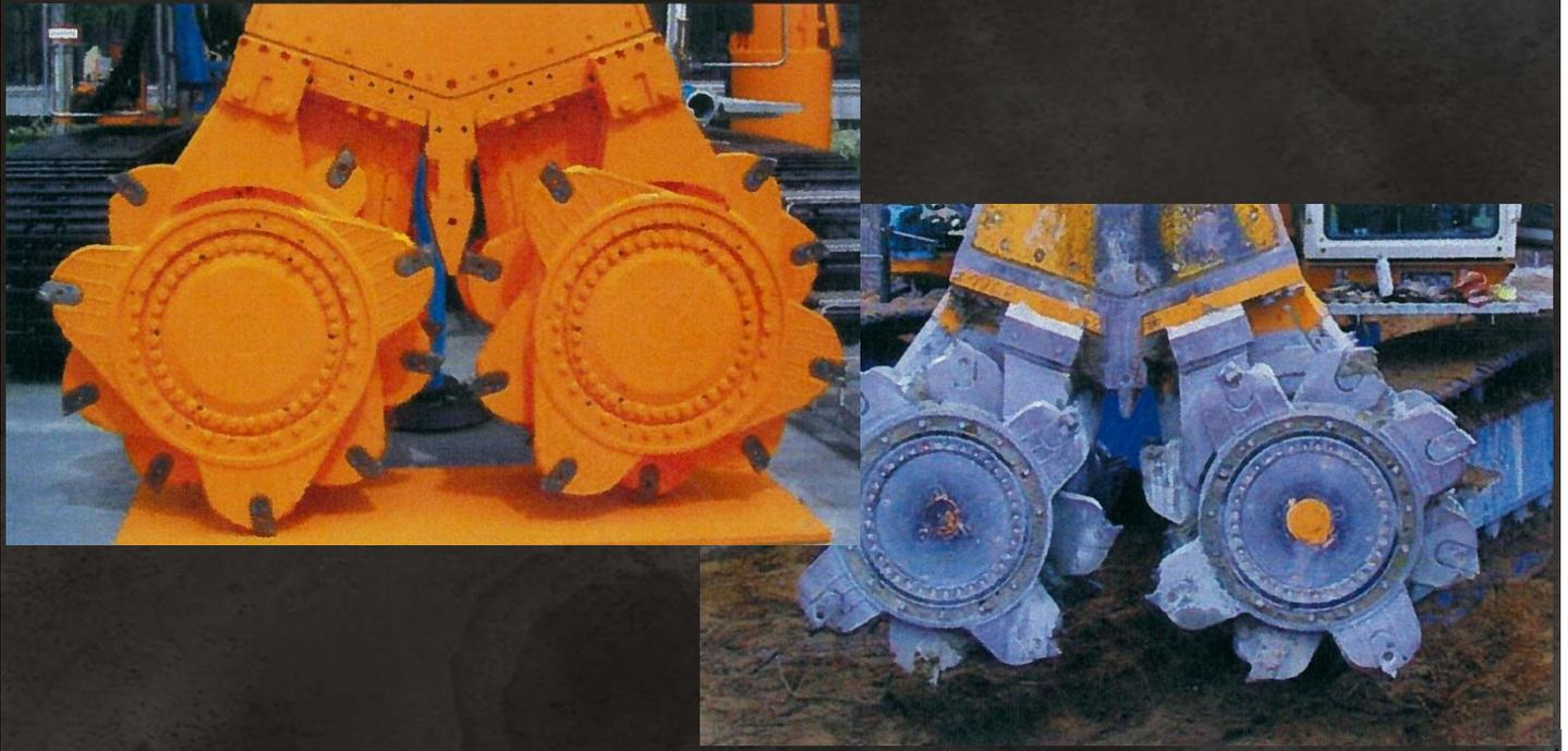
Cutter Soil Mix (CSM) technology is the latest generation of soil mixing, injecting and mixing binding agents (generally cement) with the aid of water and air with in-situ soils to produce a final hardened product. Once cured, these mixed soil/cement elements are capable of supporting soils and retaining groundwater for deep excavations, environmental cut-off walls or carrying structural loads.
