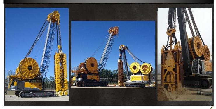
A cement-bentonite or soil-bentonite Cut-Off Wall's (COW) primary purpose is to mitigate the flow of groundwater. The COW is constructed using a trench cutter and can be installed in almost any soil conditions. The trench cutter makes 'bites' to excavate rectangular panels in the earth.
